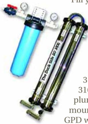
Fill your tanks with fresh drinking water from any dock with VMT's Dockside Reverse Osmosis system. Manufactured with 316SS pressure vessels, ultra low pressure high-flow membranes, corrosion resistant flow meters, 316SS pressure regulating valve, 316SS mounting hardware and plumbing, and powder coated mounting brackets. Makes up to 3,000 GPD with 100 PSI inlet pressure.
